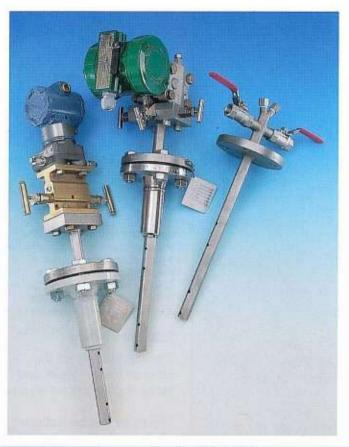
duct to measure the flow (dynamic pressure). As opposed to this, the PITOBAR averaing pitot tube has a number of holes depending on pipe size pointing towards the up-stream side. One port pointing down stream measures the static pressure.
