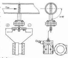
The differential pressure transmitter shall be mounted below the PITOBAR to let air escape into the main pipe line.
